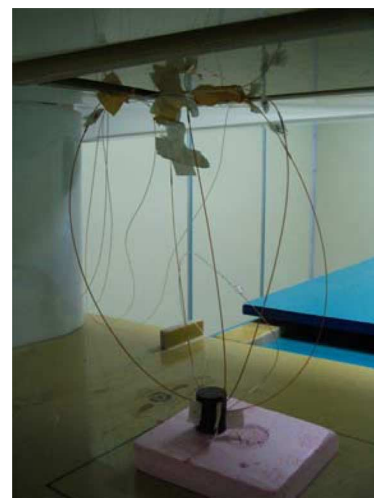
Fig. 2. Temperature Elevation Experiment: The cylindrical maghemite-gelled composite was located in the device aperture. Six optic fibers were inserted into the composite to measure the temperature. When the device power was switched on, the ac magnetic field was produced and the cylindrical composite was heated up.
