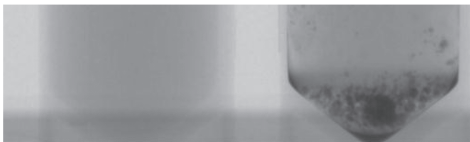
Figure 5. Micro-CT radiography of the microspheres. The left is the microspheres soaked in the n -hexane solution; the right is the microspheres soaked in the iodine n -hexane solution.
